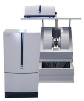
**EMXplus**Supreme Resolution and Sensitvity for EPR Spectroscopy
