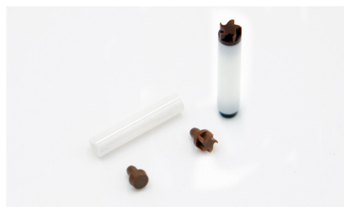
2.5mm open MAS rotor with drive and bottom vespeI caps
