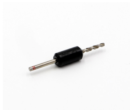
Packer: compresses sample inside rotor ( H148513 )
